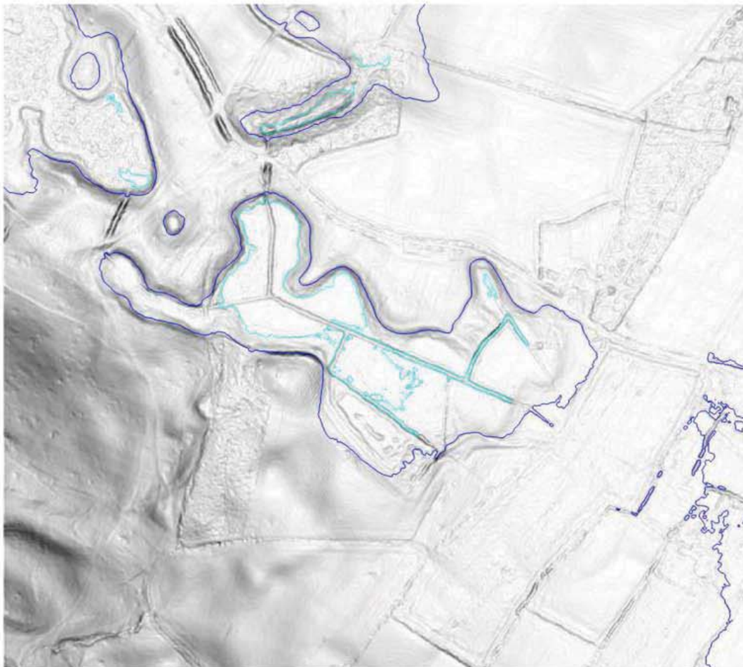
Figure 3: LiDAR slope. White to black implies slope angle from flat to 30 degrees, dark blue is the 77m contour & light blue the 75.4m contour. The area is approximately 950m wide.
