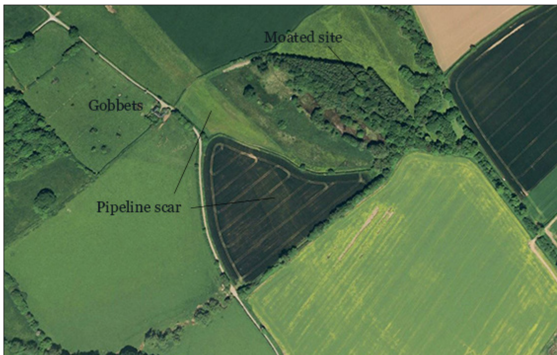
Figure 42 Google Earth image dated 24/5/2009 showing the pipeline scar – a band of different coloured vegetation caused by the gas pipeline cut passing between The Gobbets and the moated site. Google Earth accessed 16/08/2017.
